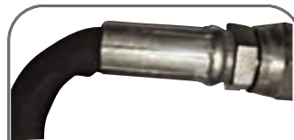
Hose bent too tight, damaged at end of coupling
