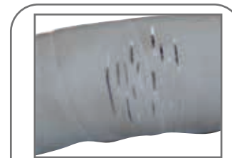
Hose with cover cracks due to age or the effects of ozone. Hose covers over time harden and should be replaced if this condition is found. (note: if boat has an ozone generator on board this could accelerate this condition)
