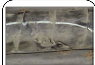
Hole in hose cover that exposes reinforcement
